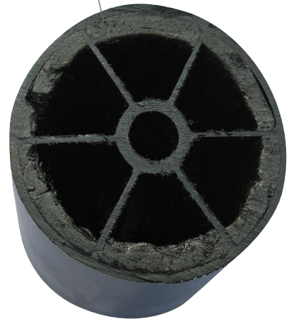
Cross-section of a 560HE rotor after a routine service interval
