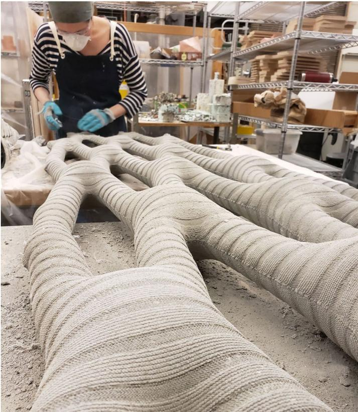
Demolding diagrid cast
